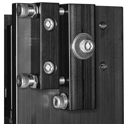
Figure 2-2. Position Screws with undersized Lock Nuts; Clamp Screws with Lock Washers; installed and tightened.
