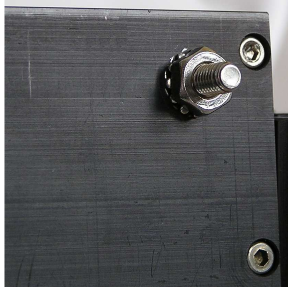
Figure 3-2. Roll Plate Lock Nut and Lock Washer Detail
